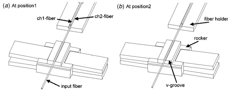
**Figure 3.** The switching mechanism.
