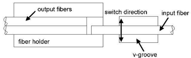
**Figure 1.** Fiber-to-fiber switch configuration.
