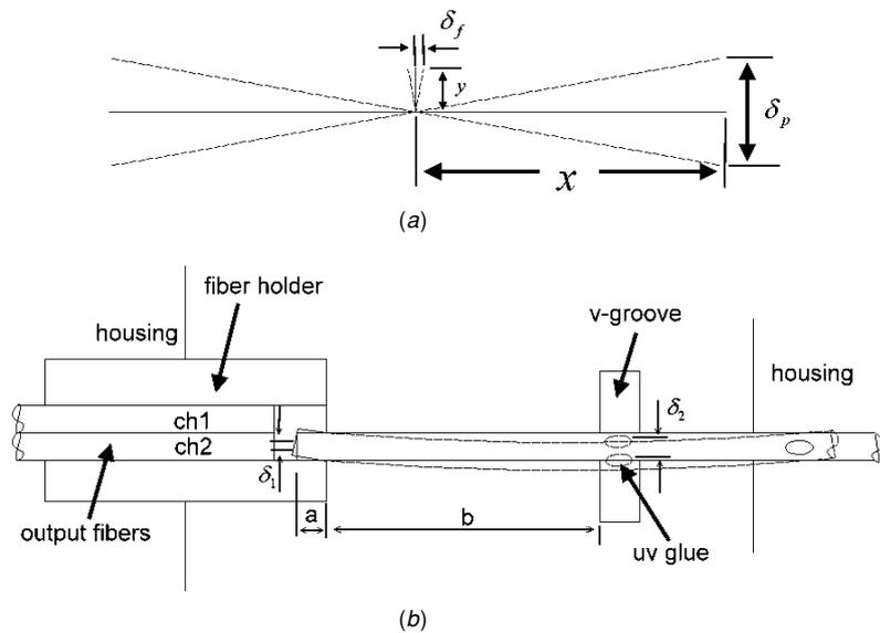
**Figure 4.** Principle of geometrical error reduction.
