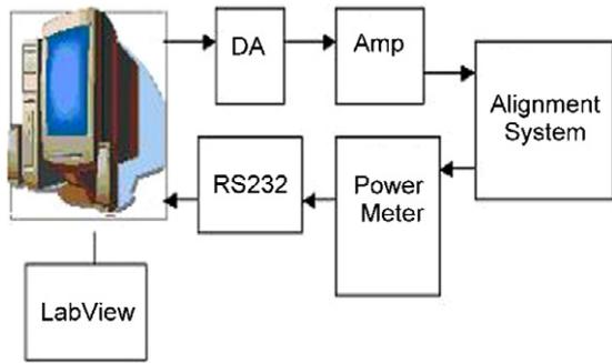
Figure 5. Block diagram of the alignment system.
