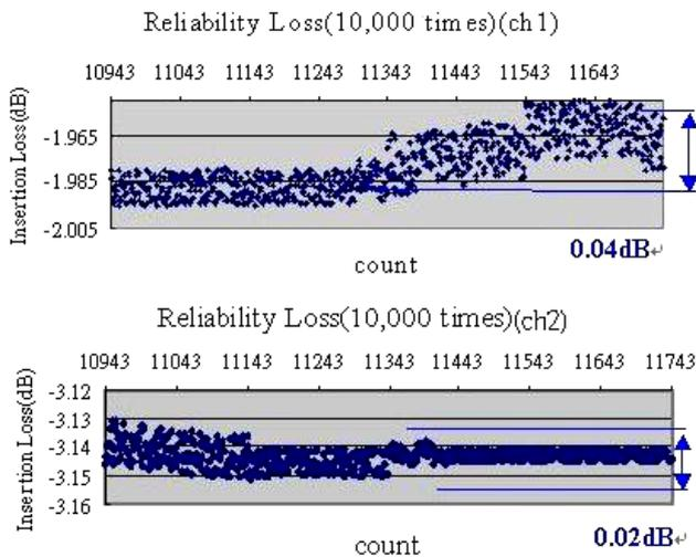
Figure 10. Reliability test of ch1 and ch2 during 10 000 cycle times.
