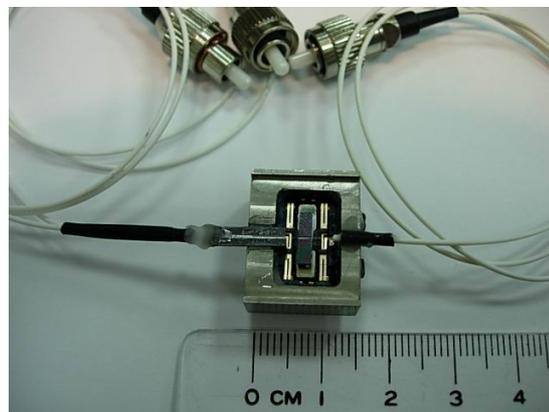
Figure 7. Photo of the developed 1 × 2 optical switch.
