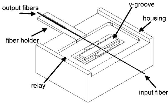
**Figure 2.** Micro/nano  $1 \times 2$  optical switch.
