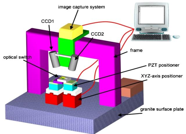
Figure 6. Experimental set-up of packaging and alignment processes.
