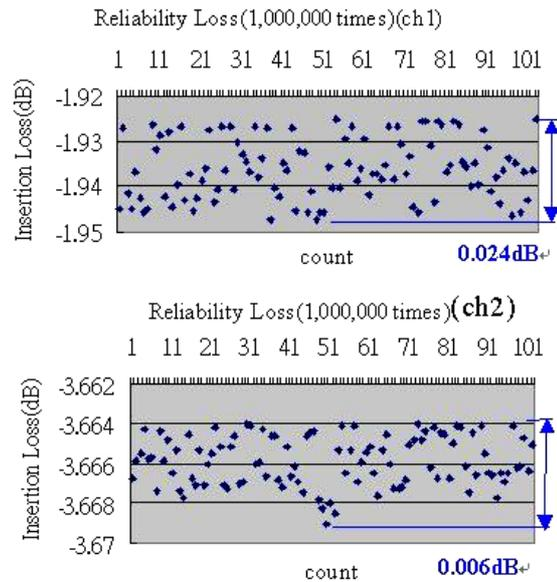
Figure 11. Reliability loss of ch1 and ch2 after 1 000 000 cycle times.
